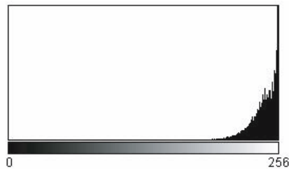
Fig. 6. Histogram describing how greyscale distributes over the pixels of the scatterplot in Fig. 2. The darker pixel has value 166. The histogram clearly indicates that a majority of pixels are pale grey.
